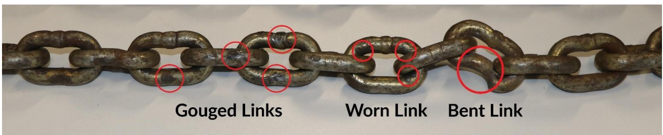
Image 2: A section of chain, with examples of wear and damage.
